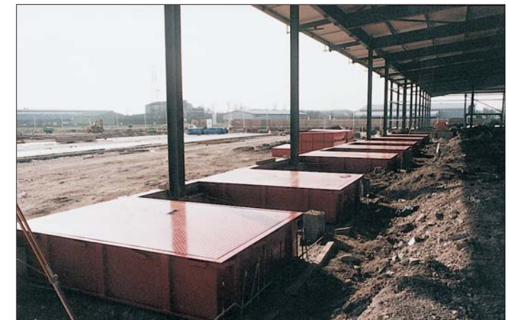
Levellers in heavy-duty fabricated steel pouring pans
